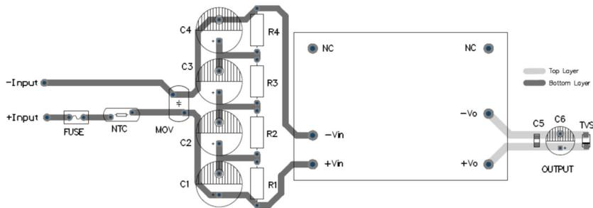
Safety and recommend wiring: line-width  $\geq 3\text{mm}$ , line-line distance  $\geq 6\text{mm}$ , line-ground distance  $\geq 6\text{mm}$
