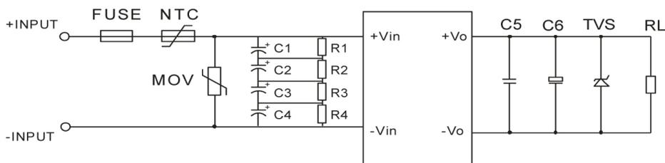
Recommended circuit for applications which require higher EMC standard (external circuit output is the same as typical application circuit)
