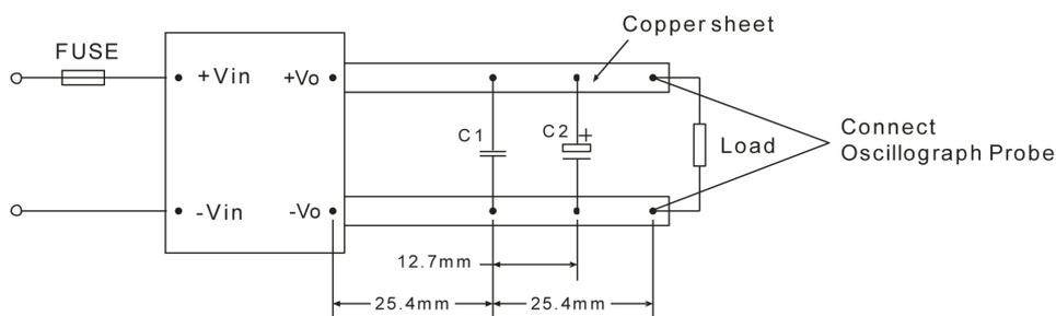
Note: C1: 1μF (Ceramic capacitor) C2: 10μF (Electrolytic capacitor)
