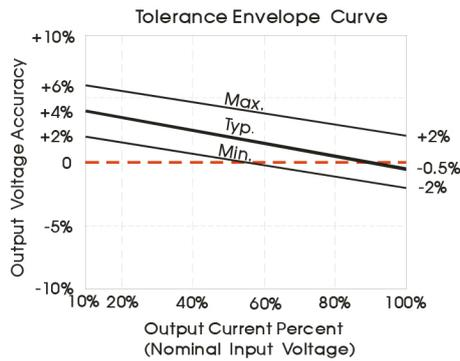
Negative Output Voltage Tolerance Envelope Graph
